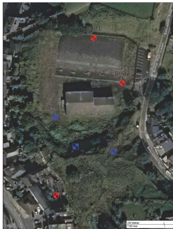
Figure 4.4: Site Investigation 2021 Exploratory Hole Plan
